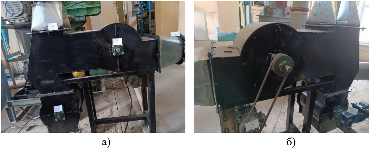
Fig. 1. Experimental prototype of the device, a catcher of large trash impurities
