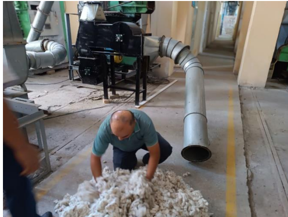
Fig. 2. Installation of the experimental setup of the large-impurity catcher device mounted in the laboratory workshop of the scientific center.
